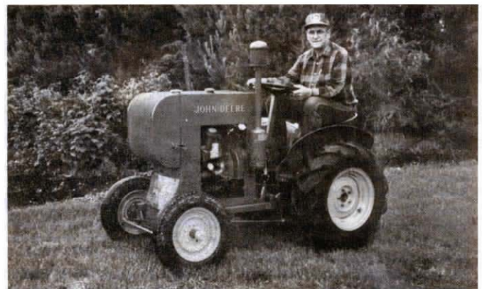
Leschasin's 25 hp miniature tractor is powered by a 2-cyl. gas engine salvaged from an old Deere 12A self-propelled combine.
