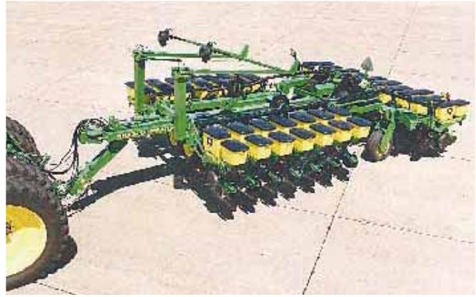
The new MaxEmerge planter features more than a dozen new improvements, including the ability to stagger closing wheels for better trash clearance.
