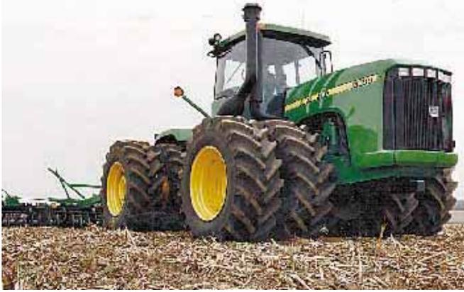
Deere's new 9400 series 4-WD tractors are powered by Deere designed and built PowerTech diesels.
