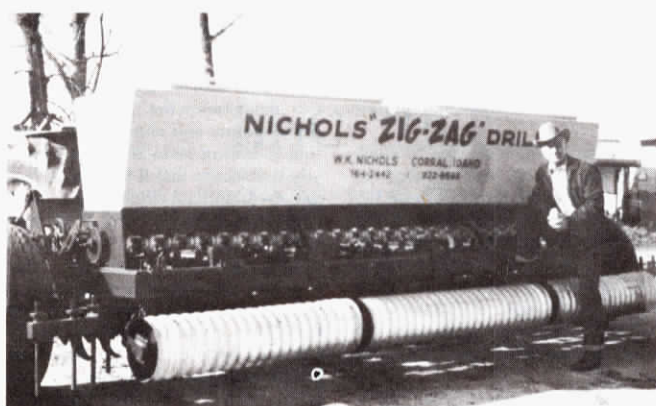
Pto-powered knives on Nichol's drill prepare a seedbed for the zig-zagging planting shoes.
