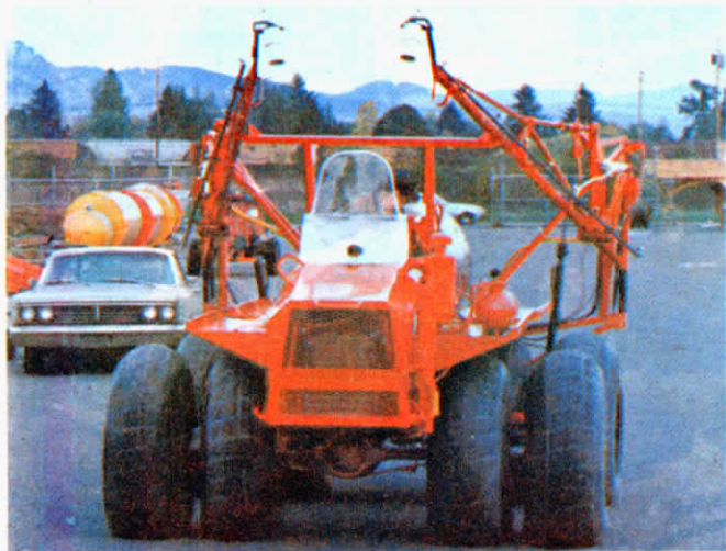
Rubber Duk's tube tires apply less than 2½ lbs. of pressure per sq. ft. of field surface area.
