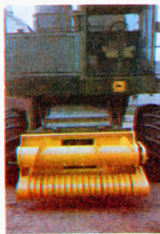
Nuehring's kit lets you mount Deere forage harvester pickup on combine for picking up windrowed oats or other small grains.
