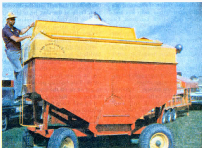
Permanent cover is 26 in. high and weighs 250 lbs. Two-section lid, shown on left, is gasketed for a rain-tight fit.
