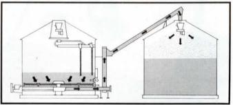
New DMC Grain Flow system augers dried grain to the center and out. Accu-Sensor unit, located in discharge auger, controls automatic removal of dried grain from the bin at predetermined moisture level. Twin augers are used for even grain flow and to equalize pull on the center gear box.
