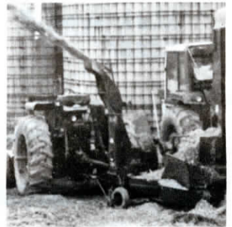
Harvester blower spout mounts upside down on silo blower.
