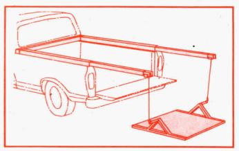
Load lifter can pick up 1,000 lbs. on its lifting platform, or load a big bale (as at left).
