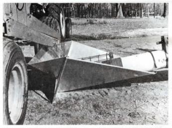
Wagon is driven alongside hopper as shown above. Alignment isn't critical since hopper folds out, as shown, to swing out and under the wagon's gravity-flow unloading chute.
