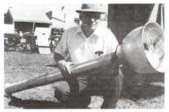
R. H. Fredericks, manufacturer, with his company's new portable aerator with auger-type end which allows the unit to be screwed into the grain without having to empty the bin.
