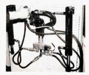
Add-on valve plugs into existing hydraulic ports with a pair of hoses and has four outlets for running two sets of hydraulics.
