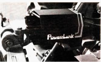
Two hydraulically-powered spur gears are turned mechanically on a screw to adjust "work angle" on the go.
