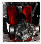
"Pump Doctor" bracket holds pump rigidly to tractor frame to eliminate bent shafts, vibration and other problems.
