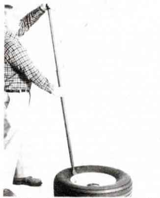
A hardened steel foot fits against the tire bead and the force of the slidehammer forces the bead away from the rim.
