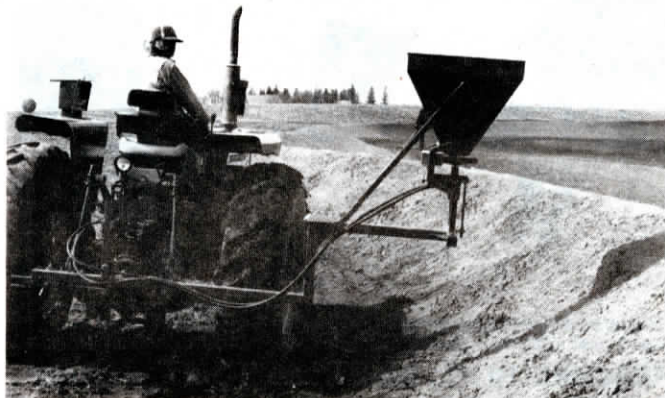
Seeder is mounted on an offset hitch attached to the tractor 3-pt., allowing Bruch to raise the seeder up and down as needed. He can vary the width of the seeding pattern by controlling the speed of an orbit motor mounted below the tank.
