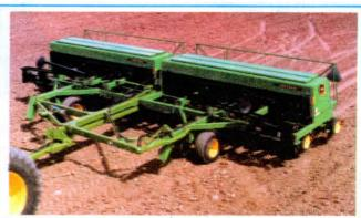
Hitch lets you pull 2 Deere 750 no-till drills. It's supported by Deere dolly wheels.
