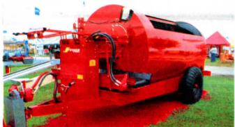
Front-mounted two-way conveyor swings out to feed from either side of mixer.
