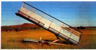
Chute (23 ft. long) is raised and lowered with hand-operated hydraulic pump.
