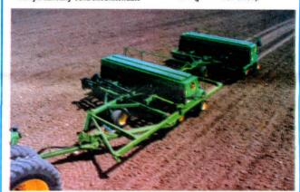
Hydraulically controlled hitch automatically moves drills into transport position.
