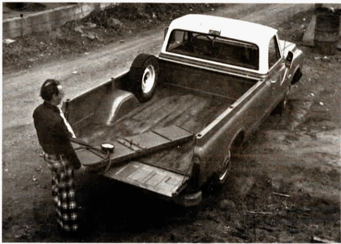
Portable scale (4.5 in. by 15 in. by 6 ft. long) has weighing capacity of up to 3,000 lbs. and can be placed in bottom of squeeze chute, or in an alleyway.
