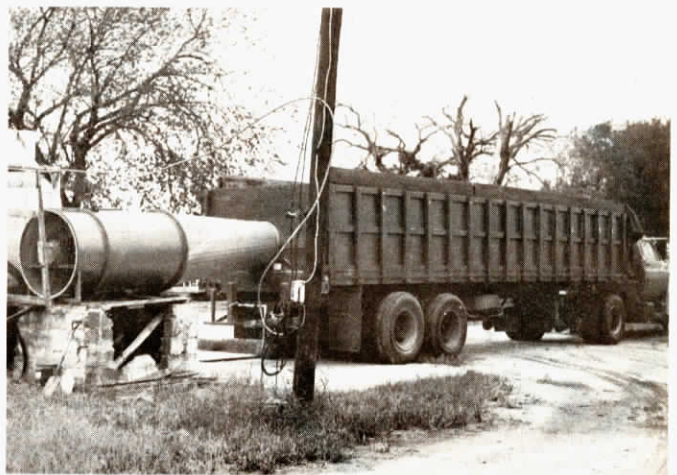
It only takes a few minutes to connect or disconnect the flexible duct-work to trucks, allowing one dryer unit to serve several trucks.
