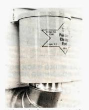
Lightweight floating cap inside outer housing rises to vent the dryer when running, then falls to close when dryer shuts off.
