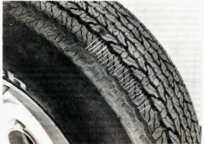
Lines drawn by artist on photo of siped tire show "sipes" — at a rate of 5 per inch — along one row of tread.
