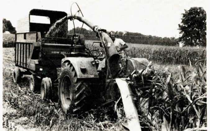
Transferring power from the turned-around tractor to the modified chopper was no simple matter, says Linde.
