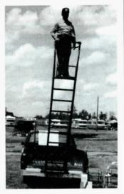
ladder has a working cage at the top. Jorgens is developing an extension ladder to use with the Porta-Perch.
