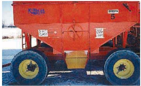
"Peel and stick" self-adhesive liner is easy to install. "Sight glass" porthole mounts ion side of box at eye level, allowing a full view inside the wagon from ground level.
