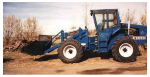
Magnuson built a 9-ft. wide bucket and mounted it on loader arms that attach to 10-ft. uprights on front half of tractor.
