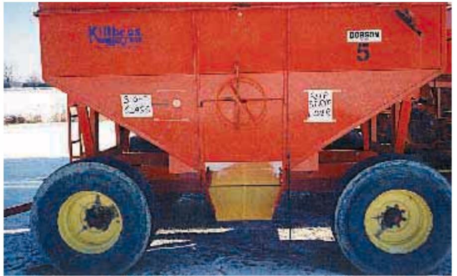
“Peel and stick” self-adhesive liner is easy to install. “Sight glass” porthole mounts on side of box at eye level, allowing a full view inside the wagon from ground level.
