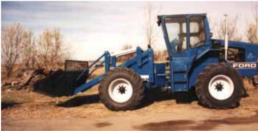
Magnuson built a 9-ft. wide bucket and mounted it on loader arms that attach to 10-ft. uprights on front half of tractor.
