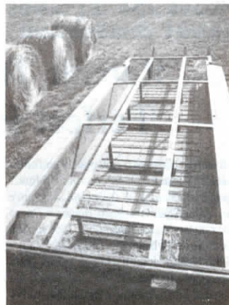
Double row of center supports made from 1 1/2-in. dia. pipe allows Krafft to stack two rows of bales across width of trailer.
