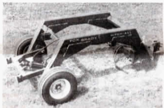
Hitch-All handles either pull type or 3 pt. equipment.
