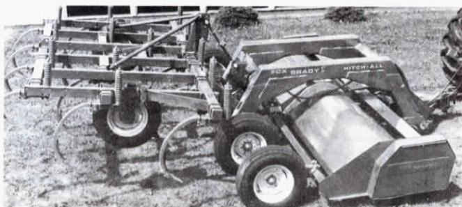
Hitch-All lets shredder operate completely independent of tillage or planting equipment trailing behind it.
