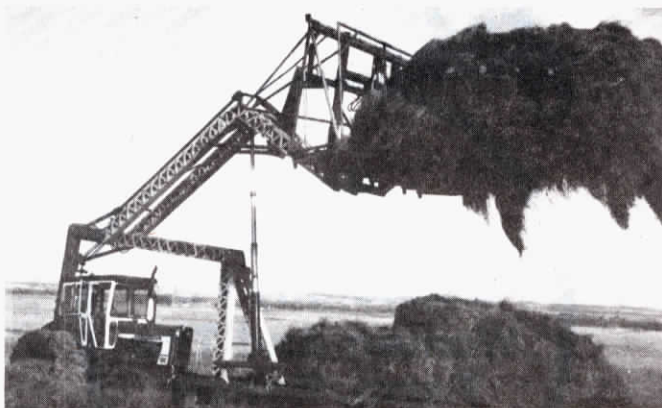
Stacker features a dolly-type frame built around a tractor but supported almost entirely on its own frame and wheels.
