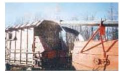
Header-mounted blower sends chopped stalks back into wagon. Rear-mounted blower delivers cobs, husks, and chaff.
