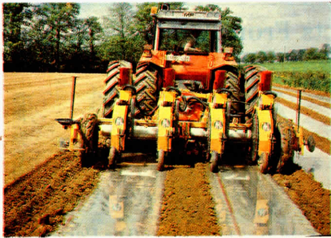
Four-row Nodet planter lays down two strips of plastic, then "punches" individual kernels through the plastic in a once-over operation.
