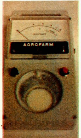
New Agrofarm tester uses ultraviolet light to determine fat content of raw or homogenized milk.
