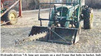
Hydraulic-driven 7-ft. long saw mounts on a steel frame that bolts to bucket. Individual sickle sections are bolted to a length of heavy-duty chain off a haystack mover.
