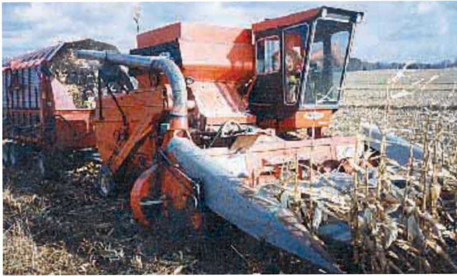
New Idea 844 4-row corn head is fitted with flail choppers, cross auger, and blower.
