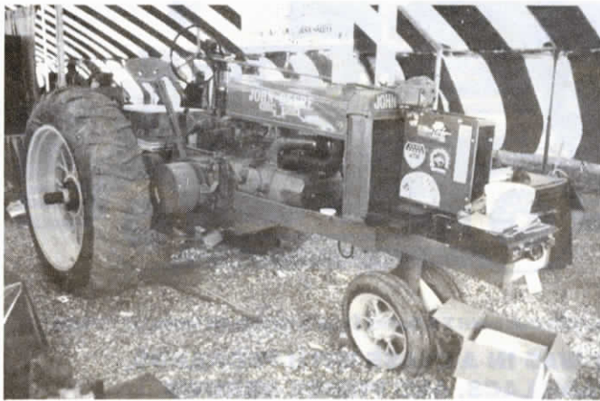
Boehler bored out the 2-cyl., 4-stroke, horizontally-mounted engine and also modified the carburetor to draw more air. Twin chrome stacks mount on top.
