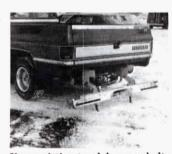
Your existing truck bumper bolts to the tire carrier, which swings down when you need the spare.
