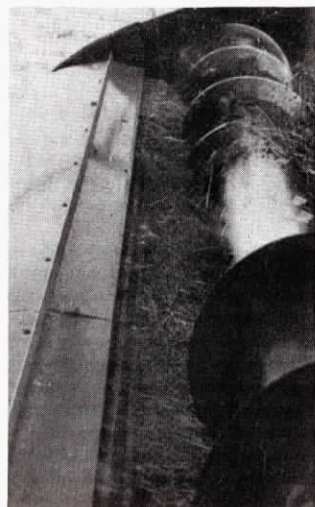
Murphy vacuum pickup sucks up shattered grain or grass seed off the ground.
