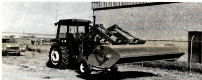
All-aluminum "stripper" (12-ft. wide) weighs only 750 lbs. and is light enough for use with 50 to 60 hp. tractors.
