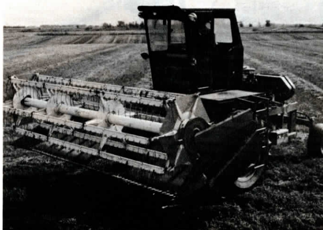
Revamped rig is "all combine" except for added-on canvass and Owatonna reel.
