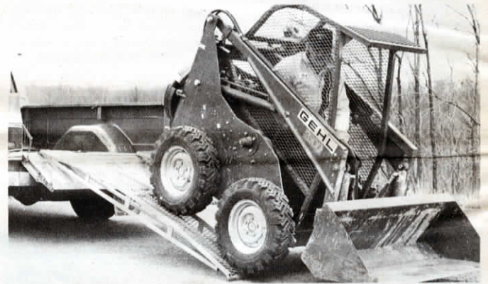
Ramps are arched in the center so low-slung equipment will clear.
