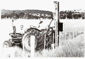
New Post Sett offers drilling and driving in one machine. It will set posts in existing fence lines and can also be used to pull posts. Without moving tractor, operator can drill a pilot hole, then swing driver into position to drive an oversized post into pilot hole.
