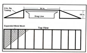
I made drive-over ramps 24 in. wide and 8 ft. long out of 2-in. thick-walled square tubing for dumping ear corn into my elevator drag line. We pull wagons with a pickup and before I built these ramps, it took a lot of time to pull up to the elevator, get out, let the drag line down, get back in the pickup, back up and then dump the corn. Then you would have to get back in the truck, pull ahead, and raise the drag line. We had to do that for
