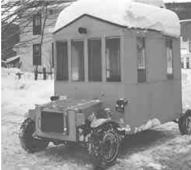
Fish house is powered by a snowmobile engine. It has a top speed of 40 mph.
