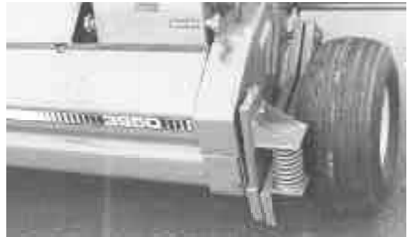
Spring-loaded flotation kit for Deere pull-type forage harvesters reduces bounce.
