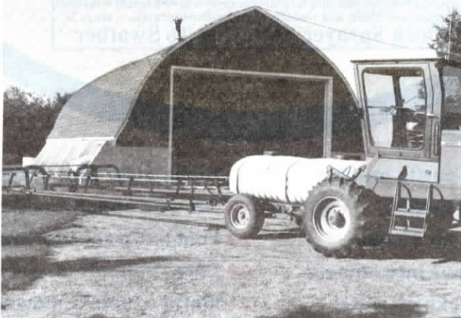
Huff likes the visibility and maneuverability of up-front sprayer as well as the fact it gives him a second job for his swather which would otherwise sit idle most of the year.
