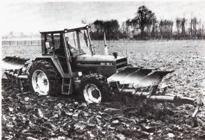
Front-mounted plow which the tractor pushes "replaces useless front ballasts with a plow that works," says the manufacturer.
