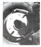
12 weights weighing a total of 1,800 lbs." In another test, he bolted a second dual wheel directly to the plate. Again, it survived the test without breaking or cracking.
