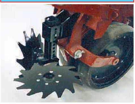
Row cleaning wheels have a concave shape and are equipped with slanted teeth that brush heavy trash out of the way.
