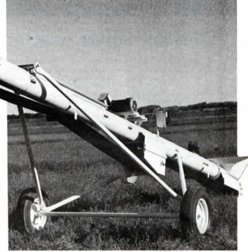
Belt conveyors (12 in. belt) available in standard lengths from 20 to 60ft.
