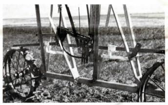
Lug Hopper attachment reduces wear at the high-wearing point of the lugs by eliminating the dragging of the trojan bar dogs over the wheel lugs.
