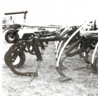
Support wheels drive an enclosed chain that turns the rod. A reverser gear can be used to turn the rod in the opposite direction of the wheels.
