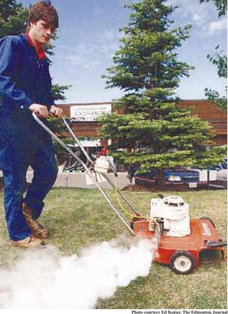
Photo courtesy Ed Kaiser, The Edmonton Journal Fogger mounts in place of muffler and connects to 1-qt. plastic supply tank on mower
