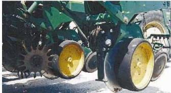
Deflector is shaped like upside down 'T' and bolts to bracket that holds the planter's Yetter trash wheels. It bends or lays stubble forward to minimize wear on press wheels.
