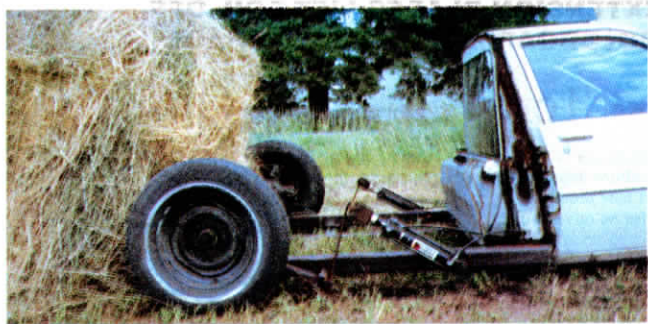
Bale carrying frame on rear of car lowers down to ground to pick up bale. A pair of cylinders pivot wheel hub assemblies up and down by pushing on a segment of leaf spring that also acts as a shock absorber.
