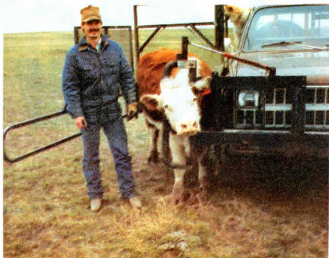
Chute attaches to front right corner of pickup. A hydraulically-activated headgate catches cattle on the run. Passenger side door can still be opened normally even with chute in place. For transport, chute folds up flat against side of pickup.
