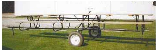
Reyhon's 20-ft. portable picnic table rides on its own set of wheels and tows behind a car or pickup. Wheels slip off each side by simply pulling a couple of pins.
