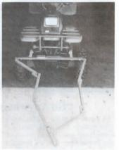
Our new Fastow folding tow bar for ATV's extends out 4 1/2 ft. for towing yet folds up to just 40 in. wide by 5 in. deep and weighs just 26 lbs. It mounts with a pair of U-bolts. When extended, the sides automatically lock in place. (Jack Horan, Fastow, Inc., P.O. Box 83, Waterville, Minn. 56096 ph 800 944-2354 or 507 362-4582)
