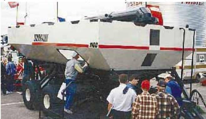
Bourgault's 1,100-bu. cart features an 18-in. dia., 15-ft. long turret auger that unloads 350 bu. per minute to either side.
