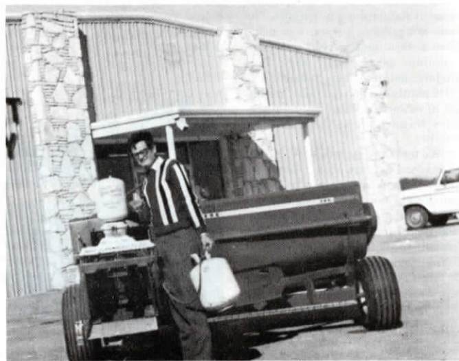
LP tanks are used to supply air pressure to the Densamatic. The device automatically controls density of individual bales.
