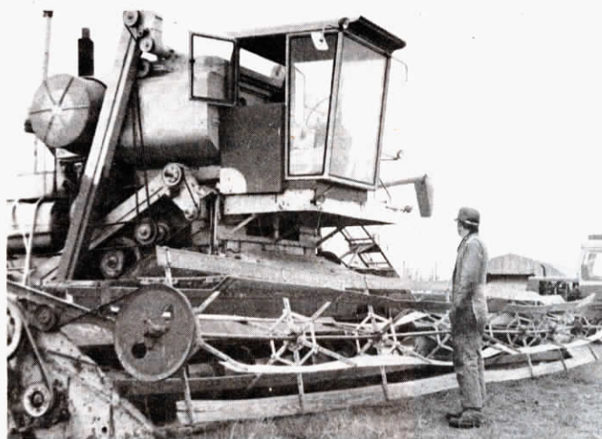
Retrofitted "Siamese" combine has 80 in. cylinder, two sets of straw walkers, 120 bu. grain tank, and 35 ft. header.
