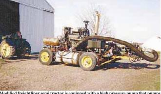
Modified freightliner semi tractor is equipped with a high pressure pump that pumps 1,000 to 1,100 gal, of manure per minute.
