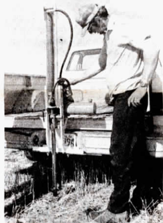
Taking a 2 ft. core sample is quick and easy with truck-mounted sampler.
