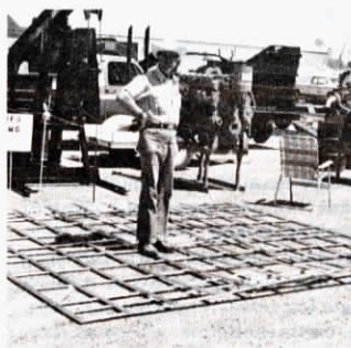
Guard flattens out so tractors, trucks and cars can drive over it without stopping.
