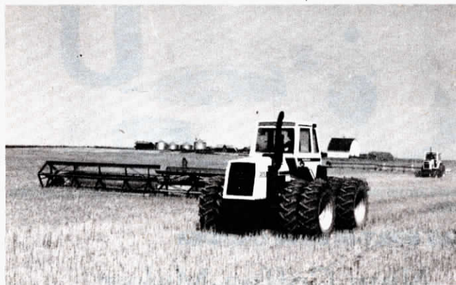
The 40 ft. swather switches from field to transport in two minutes.
