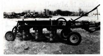
with a motorcycle wheel and odometer for keeping track of mileage when doing custom work
