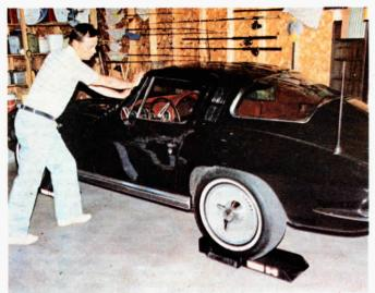
One "sideways" roller unit goes under each wheel making it easy to push a car, truck or tractor into corners of a garage or machine shed.
