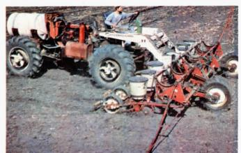
The Montags used twin screw rear ends from an old tandem axle cement truck to build the articulated tractor. It's powered by a backward-facing combine engine.
