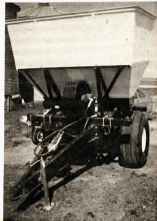
You can quickly convert cart to blow dry fertilizer either forward or backward, depending on the implement in use.
